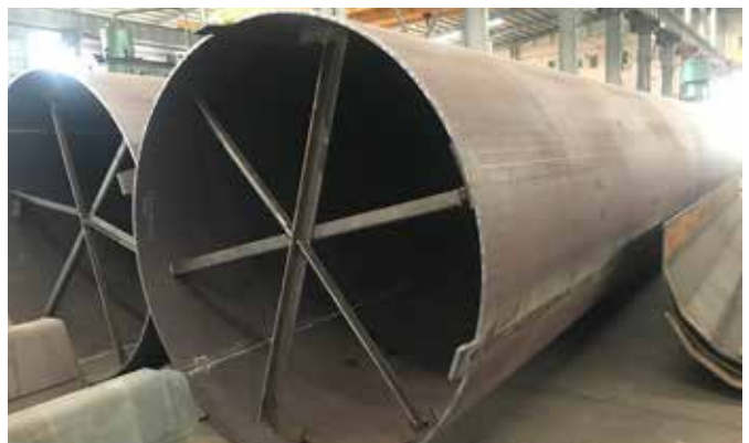
鑽探鋼管樁 Drilling Steel Pipe Pile
