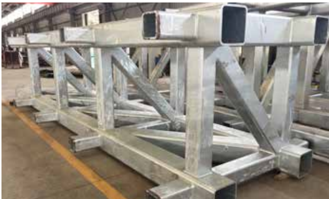
LED顯示屏鋼結構 Steel Structure of LED Panel
