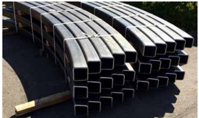
型材拉彎加工 Section Bending Process
