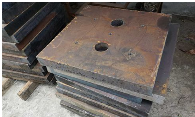
樁頭鋼板 Pile Head Steel Plate
