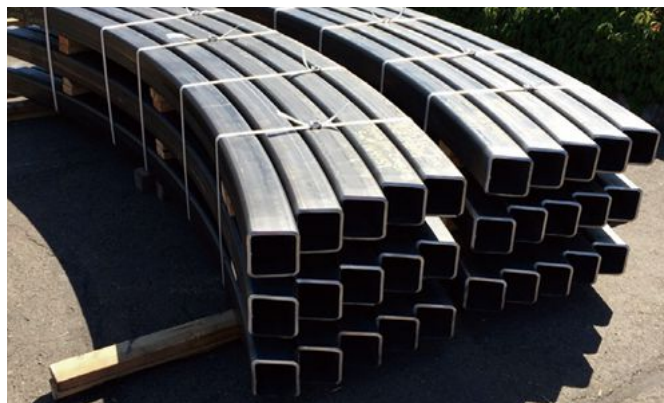
型材拉彎加工 Section Bending Process
