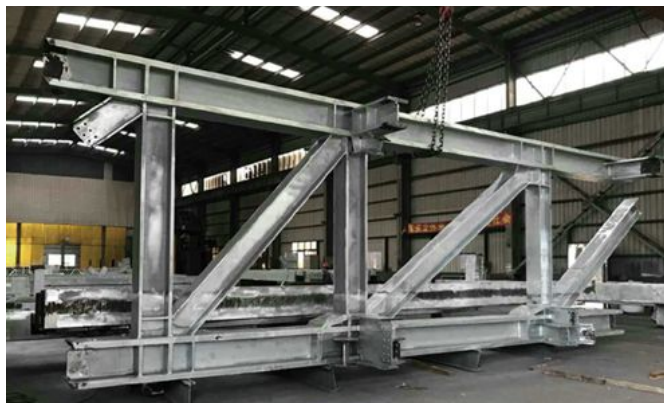
熱浸鋅桁架 Hot-dip Galvanized Truss
