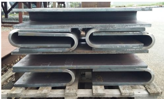
鋼板折彎 Steel Plate Bending
