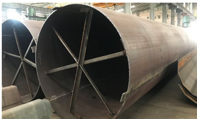
鑽探鋼管樁 Drilling Steel Pipe Pile
